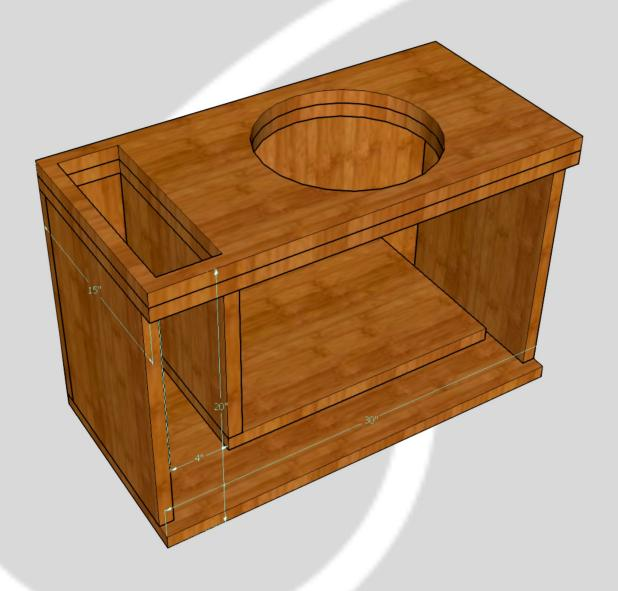
This is a 2.5 cube (70L) slot ported box tuned to 35Hz designed for good bandwidth and accuracy.
